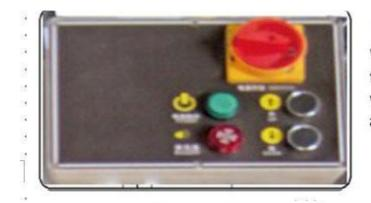
When the power supplied, turn the *POWER SWITCH* clockwise while the machine is on standby and an *INDICATOR* will show.
